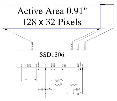
Pins connected to MCU interface: RES#, SCL, and SDA
