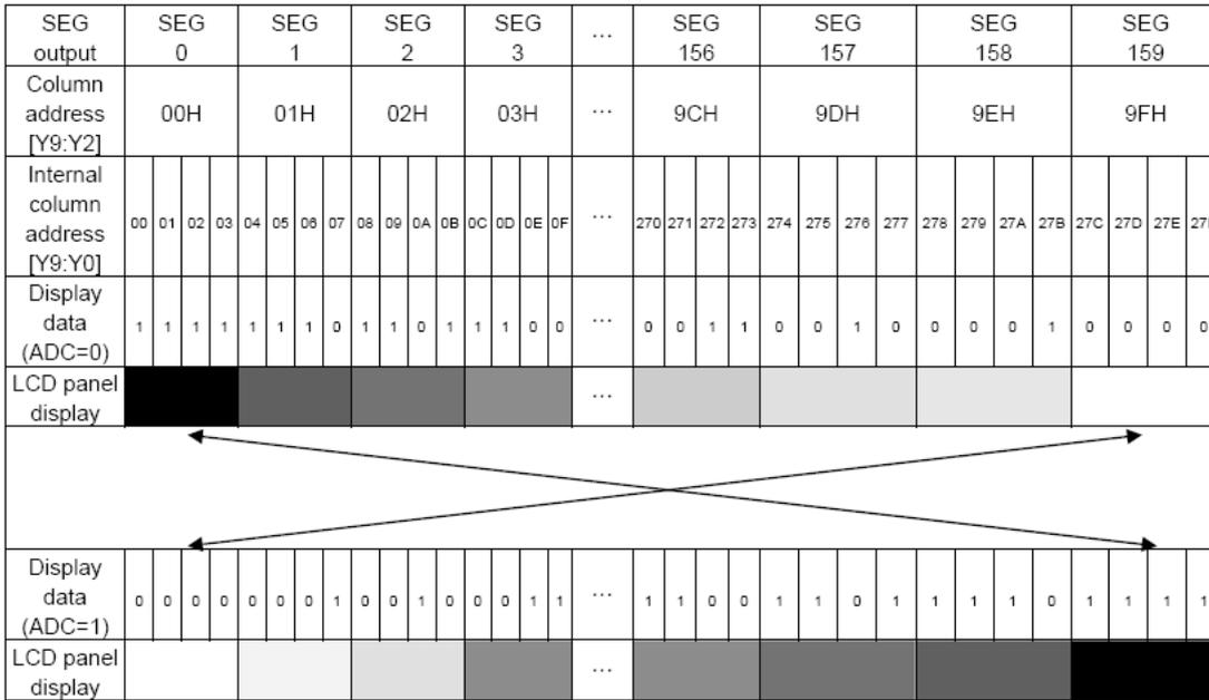
Figure 10. The Relationship between the Column Address and the Segment Outputs
