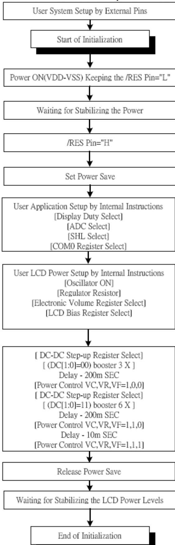
**Figure 27 Initializing without Built-in Power Supply Circuits**
