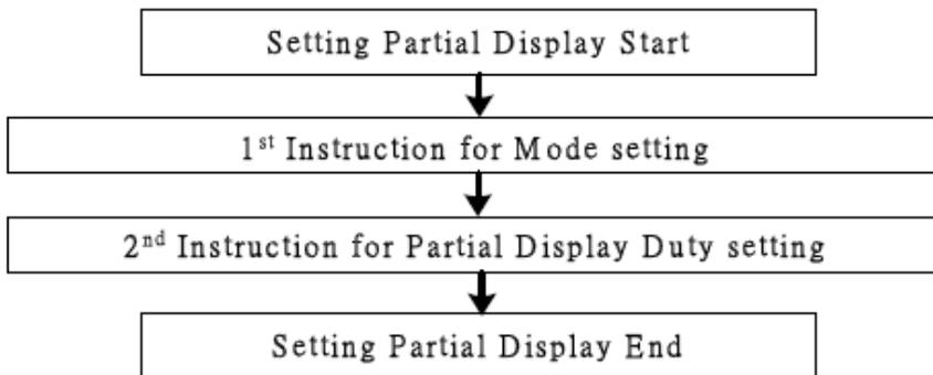
**Figure 22 Sequence For Setting Partial Display**
