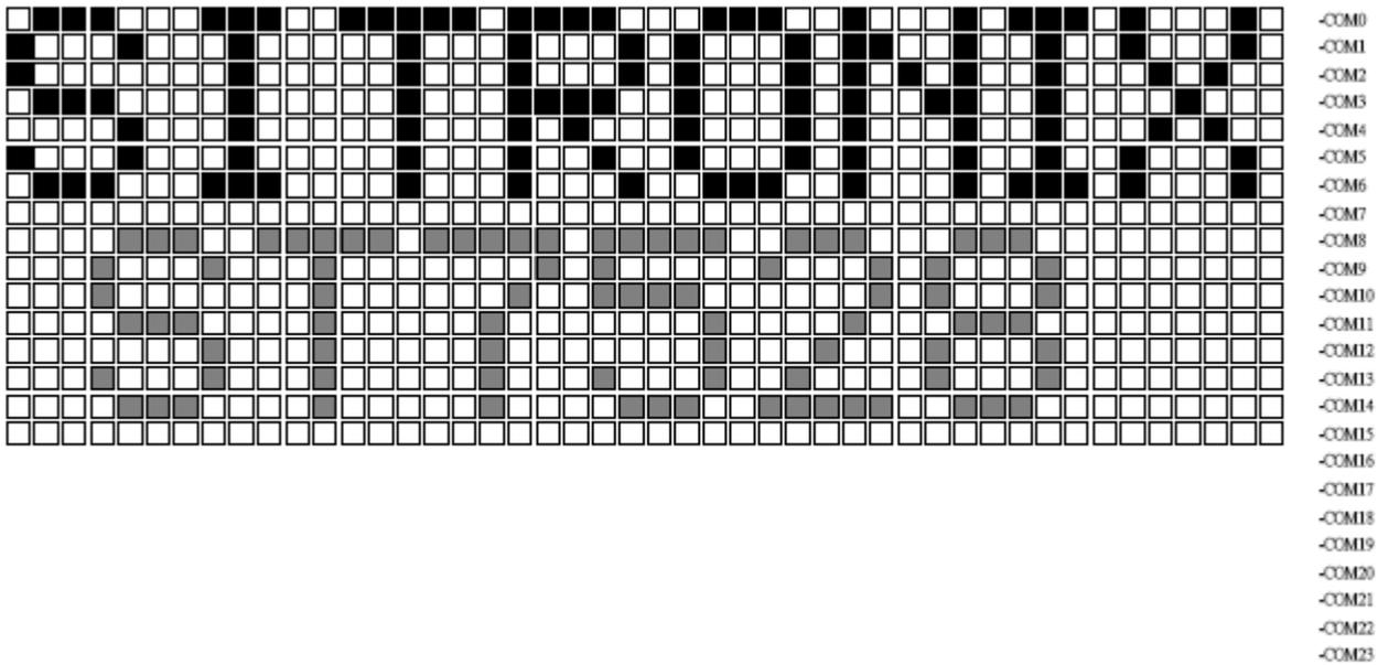
Figure 14 Partial Display (Partial Display ratio=16,initial COM0=0)
