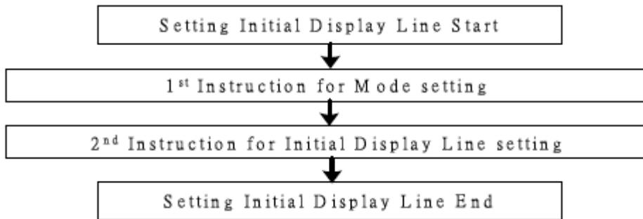
**Figure 20 Sequence For Setting Initial Display Line**
