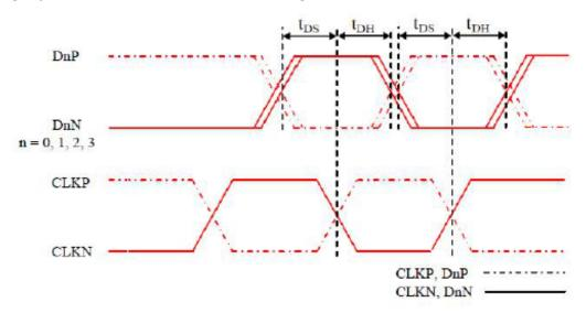
Figure 119: DSI Data to Clock Channel Timings
