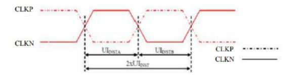
Figure 116: DSI Clock Channel Timing
