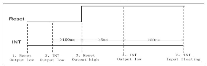
Figure 6.4: Setting Slave Address to 0xBA/0xBB Timing
