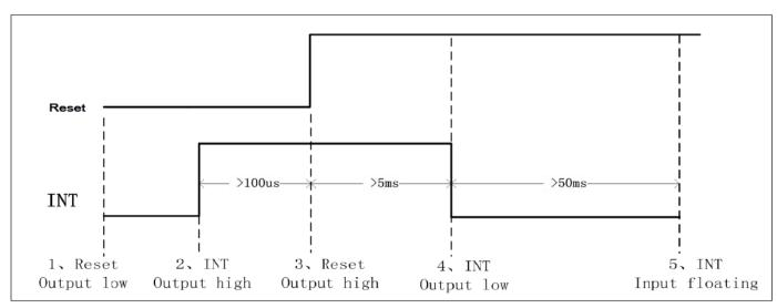
Figure 6.3: Setting Slave Address to 0x28/0x29 Timing
