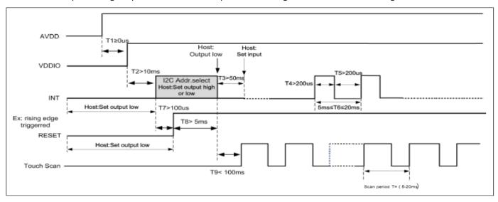
Figure 6.1: I2C Power on Timing
