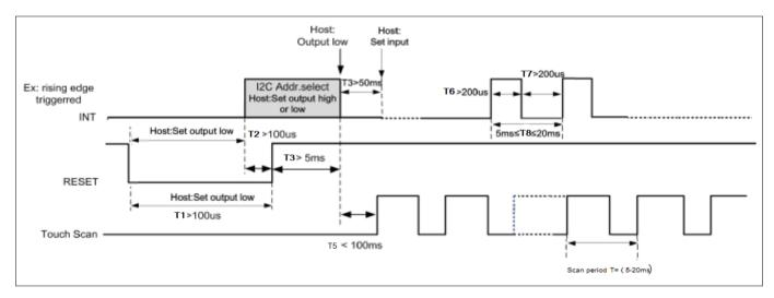
Figure 6.2: I2C Host Resetting Timing
