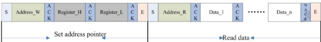
The host issues the start condition once again and sends 0xBB (read operation). After receiving ACK, the host starts to read the data. GT911 also supports continuous read operation. When receiving a byte of data, the host sends an ACK signal indicating successful reception. After receiving the last byte of data, the host sends a NACK signal followed by a STOP condition which terminates communication.
