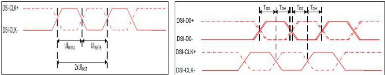
Figure 6.1: DSI Clock Channel Timing Diagram
