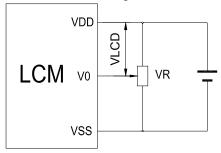
V<sub>DD~</sub>V₀: LCD Driving voltage
