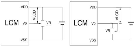
VDD~V0: LCD Driving voltage VR: 10k~20k
