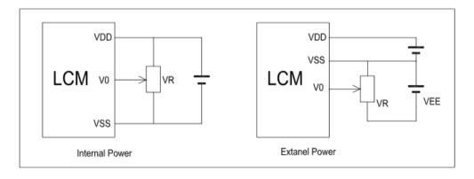
VDD-V0: LCD Driving Voltage
