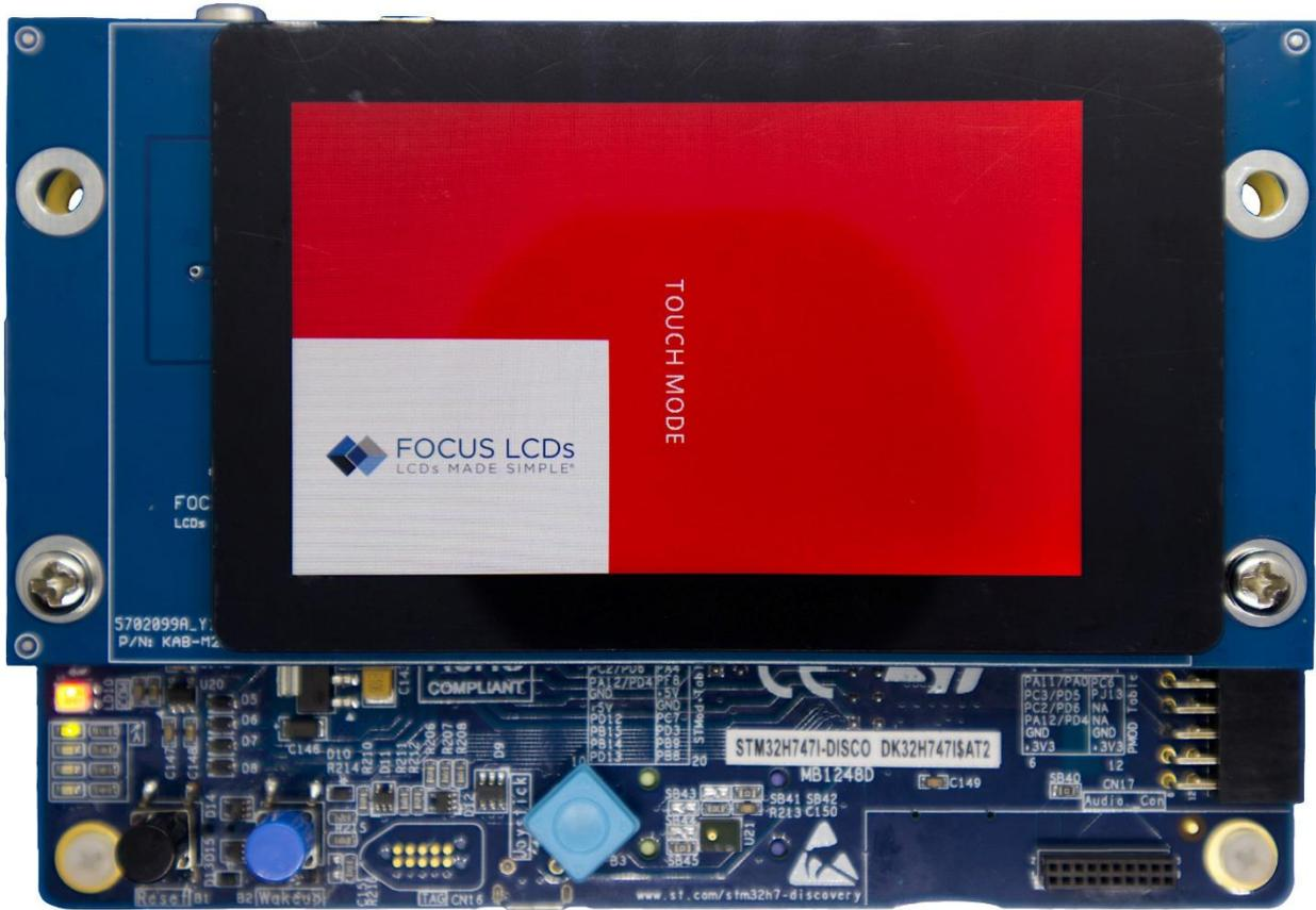
Figure 46: E35RD-MW420-C Running the Focus LCDs Demo
