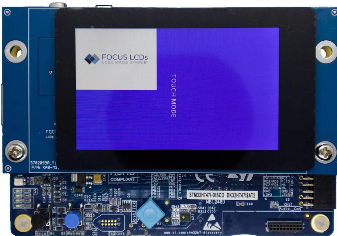
Figure 1: 35RD-MW420-C, KAB-M20SD-01 Adapter, and STM32H7 Disco Running Demo
