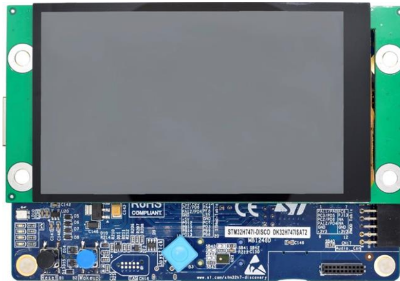
Figure 1: E43RB1-FW405-C and adapter board connected to STM32H747I-DISCO
