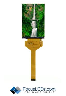
Figure 1: Focus LCDs E35KB-FW1000-N MIPI DSI Display
