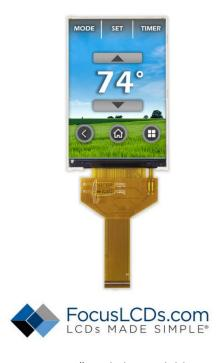
The display used in this application note is a 3.5" sunlight-readable TFT, <u>E35KA-FW1000-N</u>. This display is a transmissive TFT with 320x480 pixels and a 1000 nit backlight. The bright backlight requires 17V and 60mA to power the 10 white LEDs. Other notable features of this display are described below.
