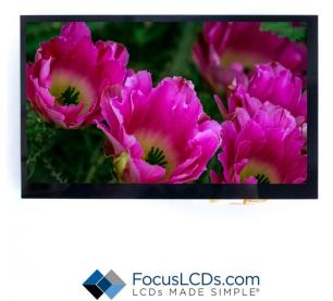
One example of a display that is connected through an LVDS interface is <u>E70RA-HW520-C</u>. This display is a 7.0" TFT with 1024x600 pixels and can display up to 16.7M colors. This display has embedded gate and a source driver IC's that can be programmed from a standard graphics controller. Below are additional features of this LVDS display.
