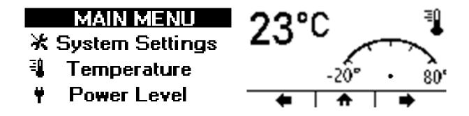
Pixel size is limited for graphic LCDs. The full page consists of 128x64 pixels so the images must be low resolution and small. The amount of RAM provided by the embedded IC of the display will support 8 full pages of display data. The images must be black and white but will appear as white and blue once uploaded to the display. Below are the images of the display with these example applications uploaded.
