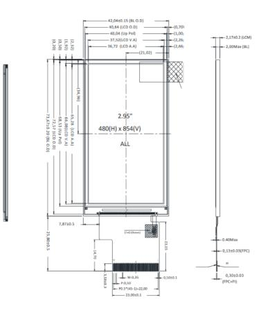
TFT displays offer a higher resolution and color depth. The TFT in this application has a resolution of 480x854 and can display up to 16.7 million colors. The combinations of color and the number of available pixels drastically increases the options for what can be displayed.
