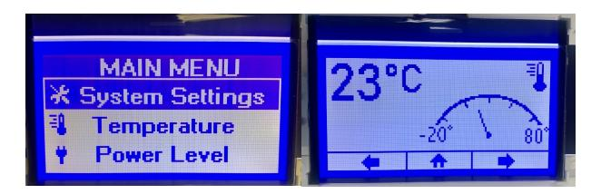
The individual pixels can be seen on the graphic LCD and can be altered to project a monochrome image. STN blue graphic LCDs will display white pixels over a blue background. The amount that can be displayed in one page is restricted to 128x64 pixels. Simple icons and characters are common options for graphic display applications.
