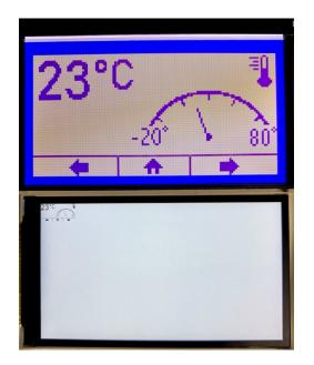
TFTs also differ from graphic LCDs because they can display colors. This display supports 24-bits of color data for each pixel. This mean there are 16.7 million colors to select from. The graphic LCD writes to each pixel as on or off. The TFT assigns each pixel 24-bits of color data which means there are 16.7M unique colors that can be displayed.
