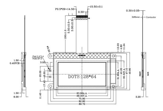
An example application for this graphic LCD will be reviewed in comparison with the TFT. The graphic LCD is interfaced over an 8-bit parallel connection. The display controller IC, ST7565, provides 8 pages of display RAM, an internal oscillator, and power regulation functions. This makes it easy to control a graphic LCD with a simple 8-bit controller because the main functions are provided internally.
