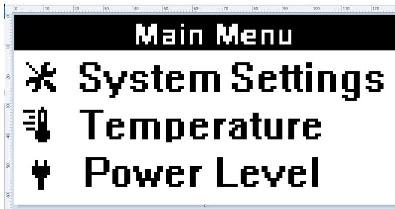
Once the bitmap is created it will need to be converted to an array of hexadecimal values to specify the on or off attribute of the pixels. The application that was used for this is called “LCD-image-converter”. There are many applications that can be used for converting bitmap images into hexadecimal, binary, and c file types.
