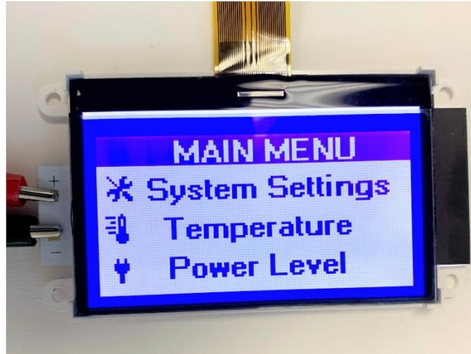
Using different pages of data can be done by specifying the page through the "Page Address Set" command. For example, a page for the menu item "Temperature" can be programmed into page 2 using the same "Page Address Set" command and writing the bitmap data into that page.
